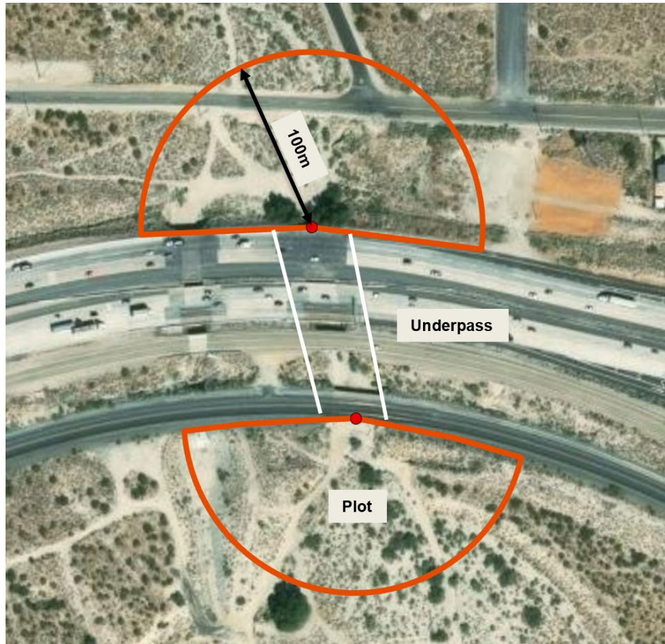
Figure 1. Example of the vegetation study plot layouts, showing the Freeway I-10, the use of the 100 m radius from the underpass, and the resulting delineated plot boundary in red. The white lines represent the underpass area.
